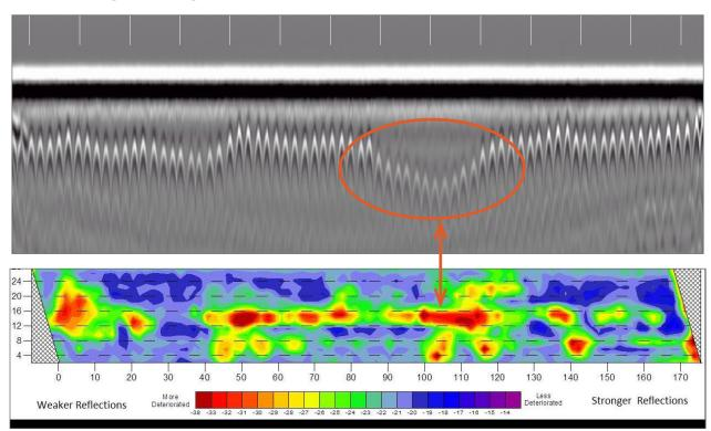
Data example on top shows the correlation between the raw data (very dim rebar) and the output to third party contour mapping software program. This shows areas of more deterioration (red, yellow..) and less deterioration (blue, light blue..)
