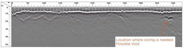
Data example above shows a road that needs further evaluation. Interfaces between layers are rugged and missing in places.
