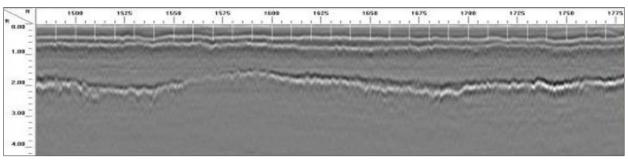
Data example above shows a road in relatively good condition. Note the clean interfaces between layers.
