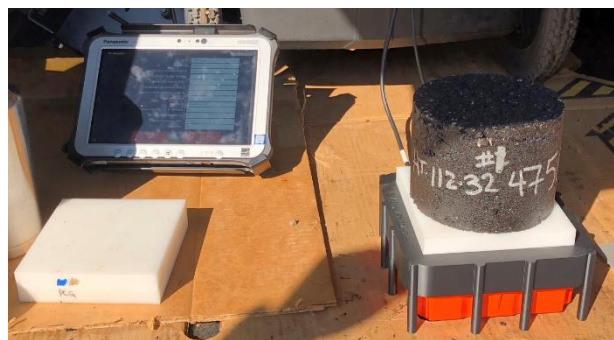
Figure 2.: An example of a field calibration method shows a puck placed on a plastic block above a GPR antenna.
