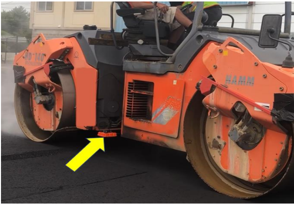
Figure 7.: This photograph shows the placement of a GPR sensor under a roller
