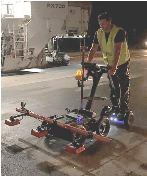
Figure 4.: This photograph shows a hoverboard linked to the back of a Pavement Density GPR. The user can safely push the cart for about 30kms before needing to recharge. This means that dense maps can be made easily and with minimal effort by the operator.
