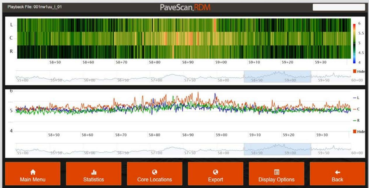
Data represents the visual output of PaveScan data. The color map indicates anomalies in the dielectric measurement. The line graph denotes the dielectric output of each sensor.
