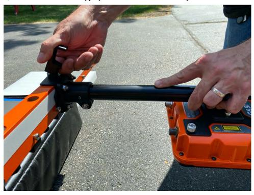
**b)** Plate must be behind stew heads when connecting the sensor boom to the bar prior to locking the latch.
