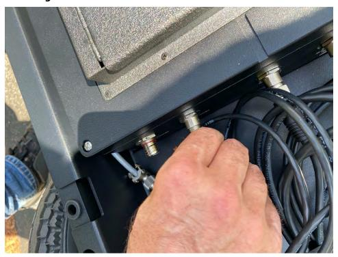
**a)** Key in and rotate to hand tighten. Guide cable through same path as survey wheel cable and up through cable management bracket and up through oval at top of handle.
