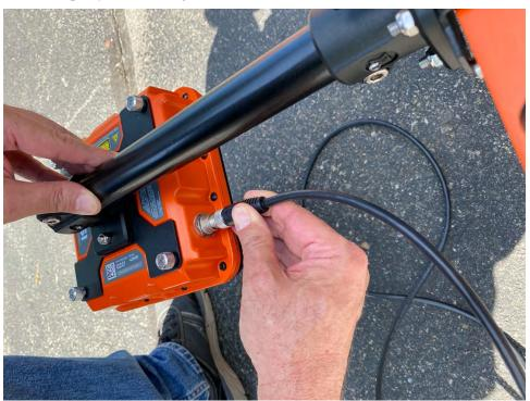
**b)** Using cable management bracket under arm guide cable through.
