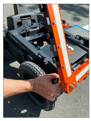
**b)** Use pull tab to unlock and unfold the arms.
