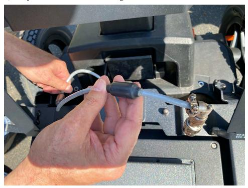
**b)** Guide the cable to the right side (facing to the front of the cart from behind the handle) of the casing, into the gap.
