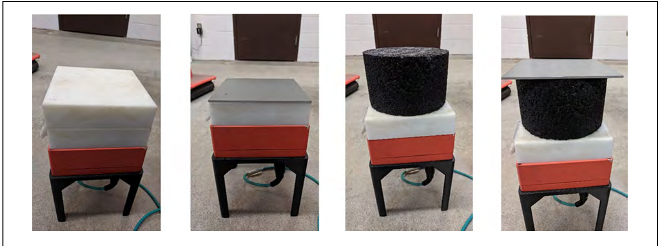
Figure 2. Experimental dielectric testing of gyratory specimens. The four setups shown in the figure are performed sequentially for 15 seconds each while operating the density profiling system to calculate the dielectric constant of the puck.
