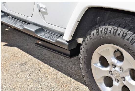
The thin 10cm ground penetrating radar (GPR) array achieves 2-3m depth penetration from a compact 12 antenna.
