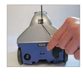
e) Insert the battery into the battery slot in back of the Mini HR. Lift the tab upward and "snap" the tab into place.
