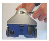
**d)** Attach the lanyard to the back of the Mini HR. The battery lanyard will attach to this lanyard to prevent the battery from falling out of the Mini HR.
