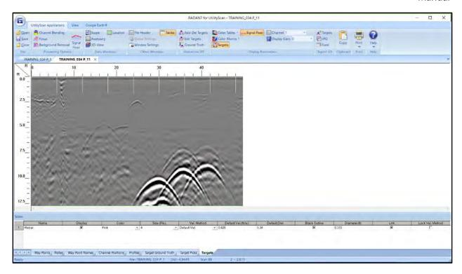
Next, press the focus button to migrate the hyperbolas. "Hmmm, I may like them unmigrated" you may be thinking. That's ok, migrate anyway after changing the slider position in the window on the left and repeatedly pressing the test and reset buttons, and then pressing the run button when you're ready to apply the correct velocity and create an output file.
