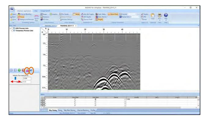
**4** Next, adjust the display channel to view all the channels of the migrated file. This is available under Window Settings.
