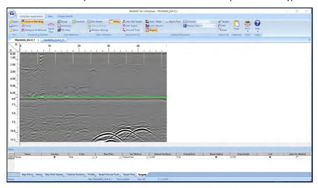
2 Click on Channel Blending. Channel blending is automatically performed (using 80% of the top channel as the blending point). The blending result is then written to both output channels. The output is a two channel file with identical data in both channels. The output file display will default to channel 1 (which you will observe by looking at the channel item in the display properties). But switching over to channel 2 will now display the same data as channel 1.
