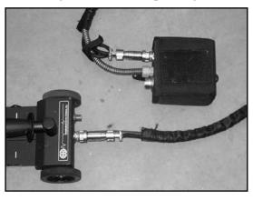
Next connect one end of the cart cable to the back of the minicart, and connect the other end to the blue padded antenna electronics box. Make sure all connections are snugged down.
