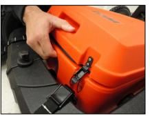
**13** Depending on site conditions and to increase the life of the capsule, you should adjust the height of the capsule by using a strap. Place a ¼ inch piece of plywood under the capsule. Loosen the straps so that the capsule sits on the plywood, and then re-tighten the straps.
