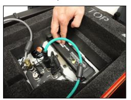
**12** Place the cover of the capsule, starting in the back as shown. Make certain there is a service loop with the cables so that there is no tension with the cables as the capsule moves up and down during data collection. Latch the cover to the locked position.
