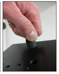
**10** If you find that the G1 is loose or that it is difficult to close the latch on the mounting unit, you may need to adjust the hex nut on the swell latch.
