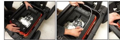
**8** Guide the green communication cable through the cable guide, through the hole at the top of the handle and connect it to the G1.
