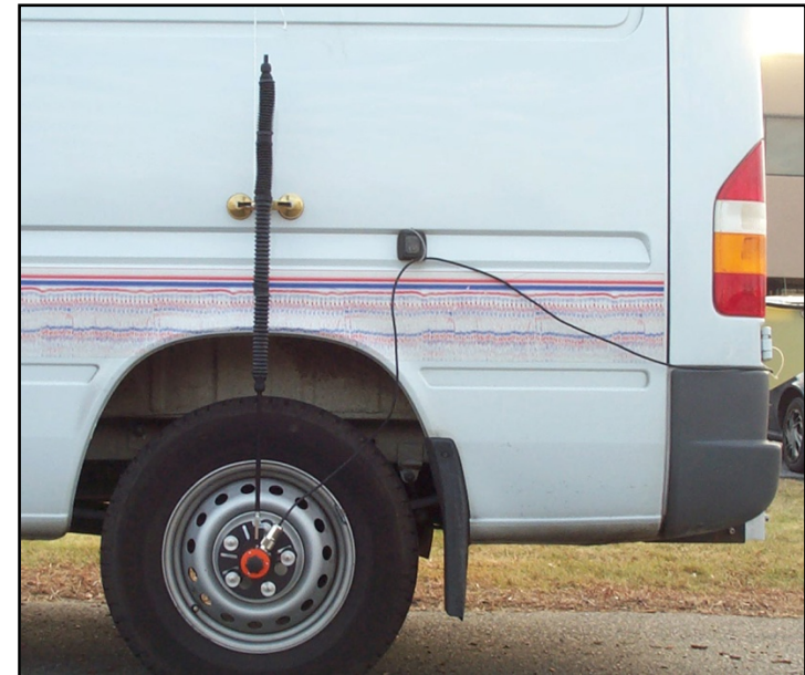
Properly assembled mount and secured cable.
