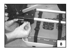
**9** Connect the female end of the control cable to port that is labeled CONTROL, connect the lead from the survey wheel (4 pin) to the SURVEY port. These leads should only be hand tightened.
