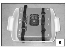
400 MHz or 900 MHz antenna, the white Velcro plate is not needed.
