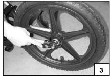
4 Ensure that the survey wheel encoder is correctly positioned on the inside of rear left wheel and that the survey wheel is making contact with the tire's rim.
