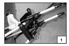
2 Squeeze the wheel-lock clamps, and insert the wheel shaft into the axle. It will slide all the way in and lock securely. To remove wheels, squeeze the wheel-lock clamp again and pull the wheel straight out. Note: The wheels are foam filled and do not require inflation.
