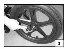
Ensure that the survey wheel encoder is correctly positioned on the inside of rear left wheel and that the survey wheel is making contact with the tire's rim.
