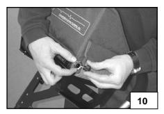
you purchased the optional sunshade, be sure that it is positioned on the outside of the bracket rather than being sandwiched between the mounting bracket and the SIR-3000.
