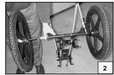
Slide the front wheel onto the front wheel fork and tighten clamp. When the clamp is slightly tight, turn the handle to the locked position. This will further tighten the clamp.
