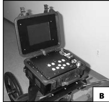
**Helpful Hint:** Placing a piece of rubber or cork between the bottom of the screen and the rest of the SIR-2000 will prevent the screen from swinging shut during survey.
