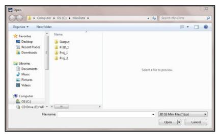
**Note:** The default file type is to open a 3D file (.bzx) collected using the StructureScan Mini. If you wish to open a 2D file, you must change the type of file you wish to open (.dzt).
