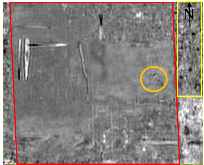
Fig. 7. Full-resolution depth slice of perpendicular polarization data 0.01 m thick centered at calculated 0.56 m depth. The pit outline is indicated by the red lines.
