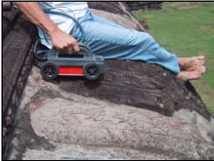
Figure 3. GPR search head was rolled over the ridge of each scanned naga to investigate subsurface conditions.
