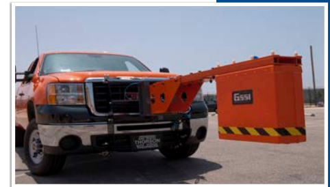
Vehicle-mounted RoadScan system integrated with FWD.
